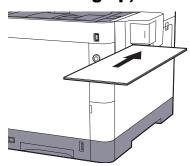
When the paper is inserted all the way in, stapling takes place.
