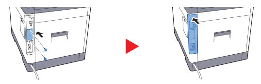
6 Insert the power cord into the socket and turn on the power switch.
