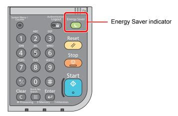
If print data is received during Sleep, the machine automatically wakes up and starts printing.
