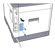
4 Insert the SD/SDHC memory card into the SD/SDHC memory card slot.
