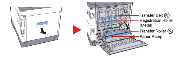
Wipe away the paper dust on the registration roller and the paper ramp using the cloth.
