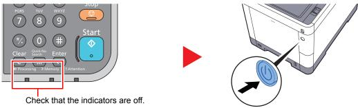
In case of not using the machine for an extended period of time...
