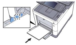
Insert the paper along the paper width guides into the tray until it stops.
