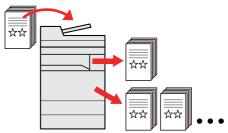
It is possible to copy one sheet before copying a large number of sheets. This enables you to check the contents and finishing and copy the desired number of sheets without scanning the original again if you are satisfied with the result. If you want to make changes, you can change the settings and copy only one sheet again.
