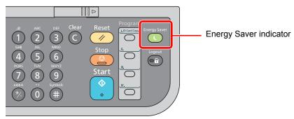
If print data is received during Low Power Mode, the machine automatically wakes up and starts printing. Also when fax data arrives while the machine is in Low Power Mode, the machine automatically wakes up and starts printing.
