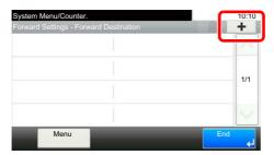
Display the add destination screen and follow the procedure below to register the forwarding destination. Only one destination can be registered.
