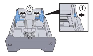
2 Adjust the paper length guide to the paper size required. Press the paper length adjusting tab and slide the guides to the paper size required.
