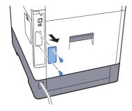
4 Insert the SD/SDHC memory card into the SD/SDHC memory card slot.
