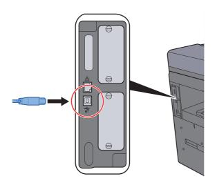
2 Connect the other end of the cable to the PC.
